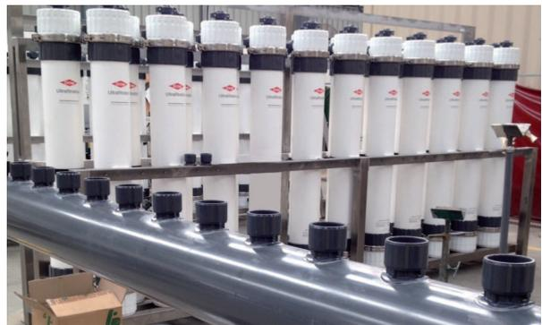
Water Treatment: The flexibility of use and simple installation makes the TP DV0 saddles a good solution for water treatment applications (in the picture a prefabrication phase of a desalination plant).
